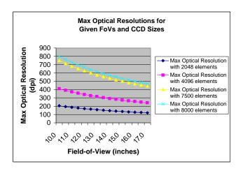
If 400 dpi resolution is required, then the maximum transport speed is (10,000 scans per second)/(400 scans per inch) = 25 inches per second (ips). This assumes that the 10.24" FoV is sufficient for the application. But what if it isn't?
